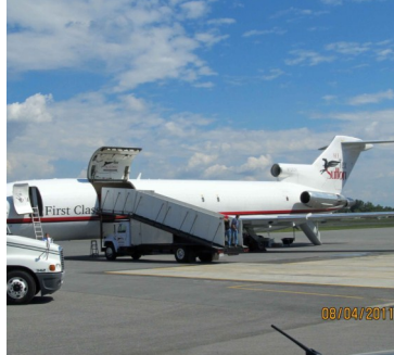
Tex Sutton's B727 customized for horse transport, sets up to offload Turbulent Descent to a van at Albany, New York.
